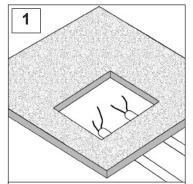
Determine box location and position in accordance to floor plan. Make a 12 3/4" (324 mm) by 8 15/16" (227 mm) cutout on the floor.
