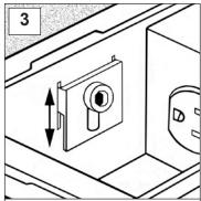
Drop the box on the floor cut out and adjust the position of the toggle until the box is secured to the floor. (See Fig A below)
