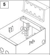
Barriers must be installed when placing line and low voltage devices on the same side of the box.
