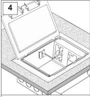
Fasten the Allen screws using a 5/32 allen wrench until the box is securely anchored to the floor. NOTE: For floor thicknesses from 1 - 1 1/4" remove the allen screw, rotate toggle 180° and install the toggle back in place.
