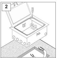
Pull 3/4" or 1" trade size flexible conduits through the floor cutout and attach them to the selected knockouts using conduit fittings. Attach the cover to the box using the four supplied screws
