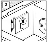
Drop the box on the floor cut out and adjust the position of the toggle until the box is secured to the floor
