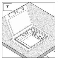
Attach devices to faceplates and secure them to the mounting panels.
