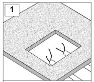
Determine box location and position in accordance to floor plan.
