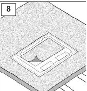
Install the desired floor covering material on top of the lid -if applicable-
