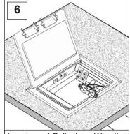
Locate and Pull wires. Wire the devices in accordance to the NEC.
