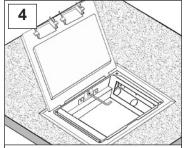
Fasten the Allen screws using a 5/32 allen wrench until the box is securely anchored to the floor. NOTE: For floor thicknesses from 1 - 1 1/4" remove the allen screw, rotate toggle 180° and install the toggle back in place.
