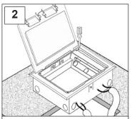
Pull 3/4" or 1" trade size flexible conduits through the floor cutout and attach them to the selected knockouts using conduit fittings. Attach the cover to the box using the four supplied screws.
