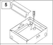
Barriers (sold separate) must be installed when placing line and low voltage devices on the same side of the box.
